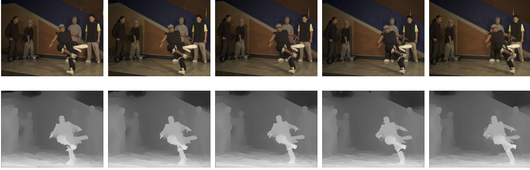
Figure 2.8: Example of MVD format with 5 views and corresponding depth maps.
