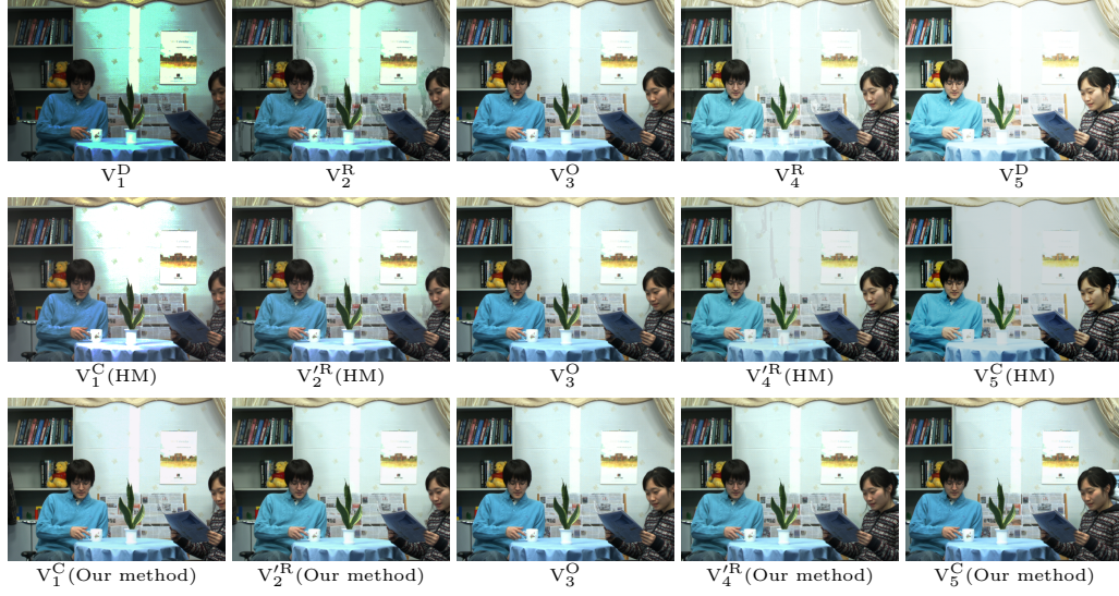
Figure 3.23: Rendering results for Newspaper sequence (top: No correction, middle: HM method, and bottom: Our method). V_i^* : View i , V_*^O : Original view, V_*^D : Distorted view, V_*^C : Corrected view, V_*^R : Rendered view before correction, V_*'^R : Rendered view after correction.
