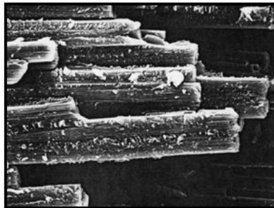
Figure II.6 : Rupture de fibre [45]
