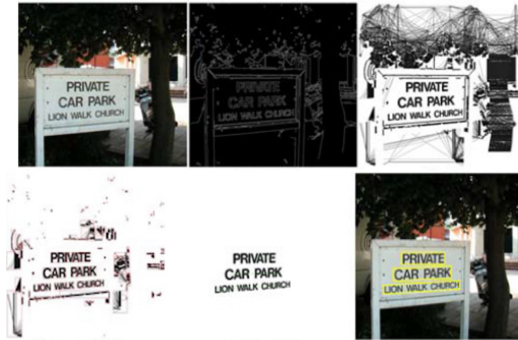
Figure 1.2: (a) Original image; (b) Edge detection; (c) SWT; (d) Component filtering; (e) Interpretation; (f) Detected texts.
