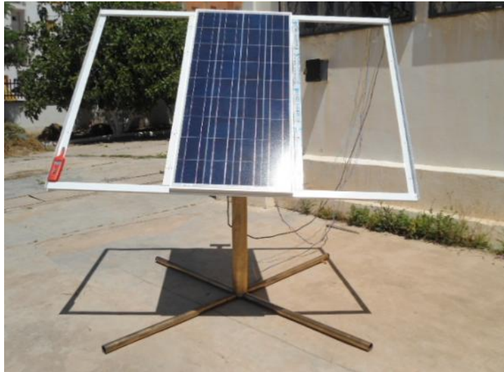
Figure 4.10 : Structure de support
