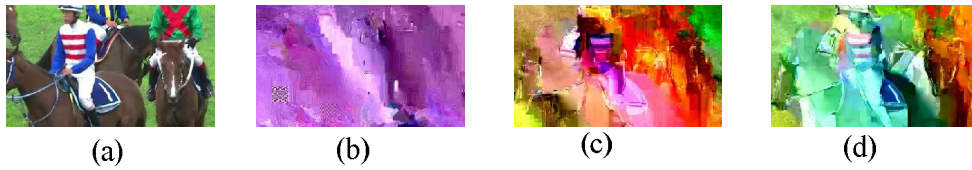
Fig. 9. Sensitivity of the proposed SE against known plaintext attacks : (a) original frame of RaceHorses sequence encoded in low delay mod,(b) attacked result at QP=18 with PSNR(Y)=7.15,(c) attacked result at QP=28 with PSNR(Y)=15.28,and (d) attacked result at QP=34 with PSNR(Y)=16.05
