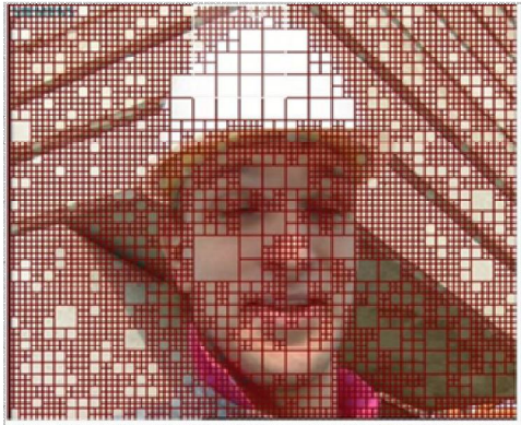
Fig. 2. Transform units TUs ranging from 4×4 to 32×32 of encoded foreman sequence in low delay mode at QP=18
