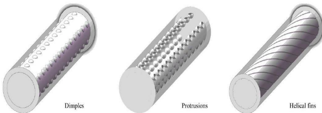
Figure II.17: Dimples, protrusions and helical fins
