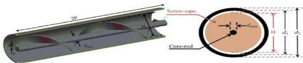
Figure II.16: Helical screw-tape inserts
