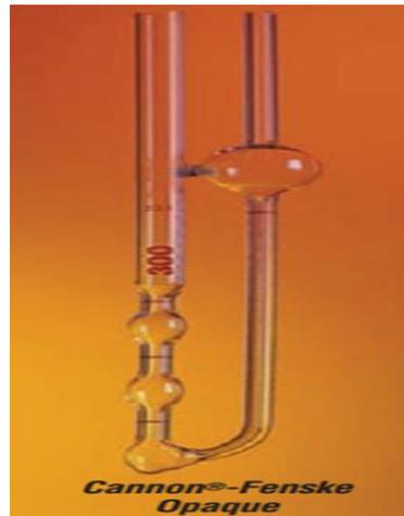
Figure II.13. Viscosimetre Cannon –Fenske Opaque
