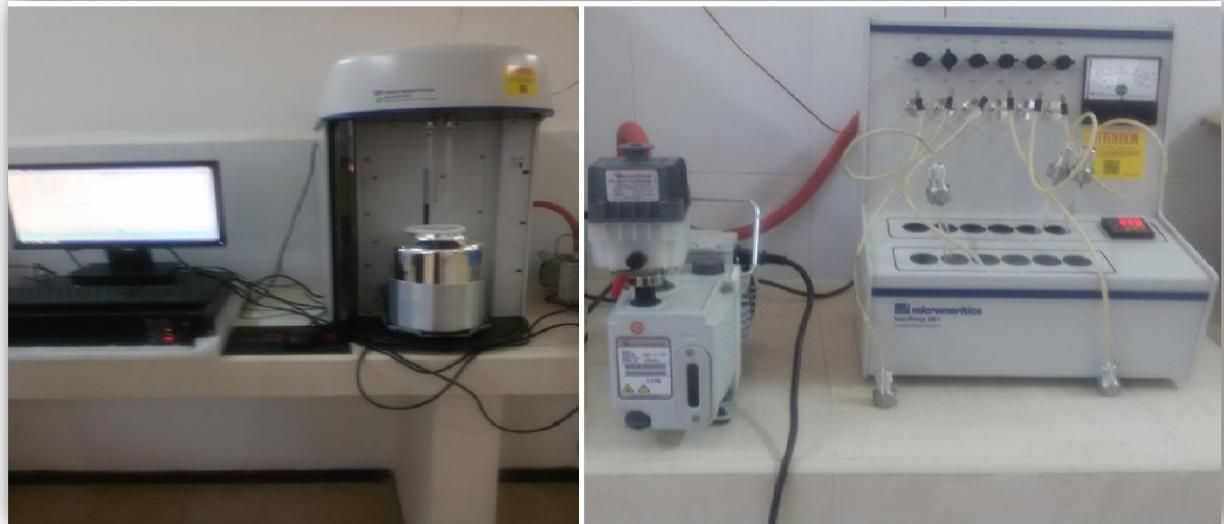
**Figure.II.10.** Appareillage de BET (Micrometrics ASAP 2000)
