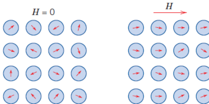
Figure 3.4 The alignment of atomic magnetic moments for a paramagnetic material with and without a magnetic field.
